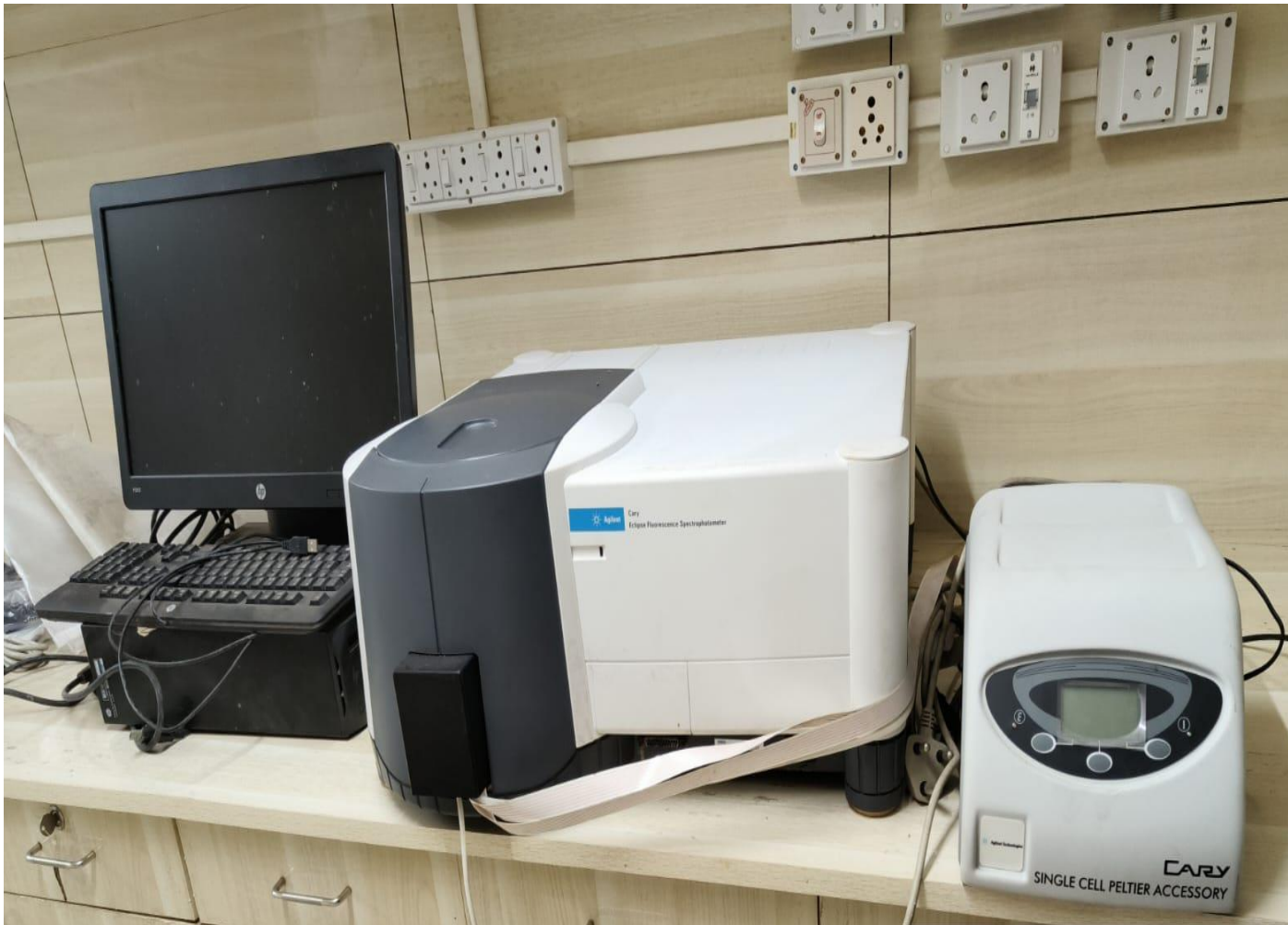
SPECTRO FLUORIMETER (DST-FIST FUND) Used to measure fluorescence spectra
